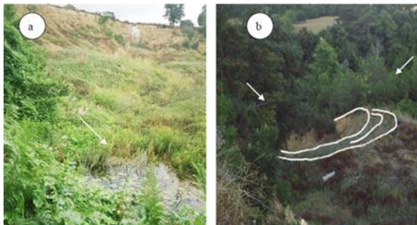
Figure 1. a) Uçuk landslide and its lower puddle, b) Curved rupture surfaces of the landslide the landslide and bends in the surrounding trees [1]
