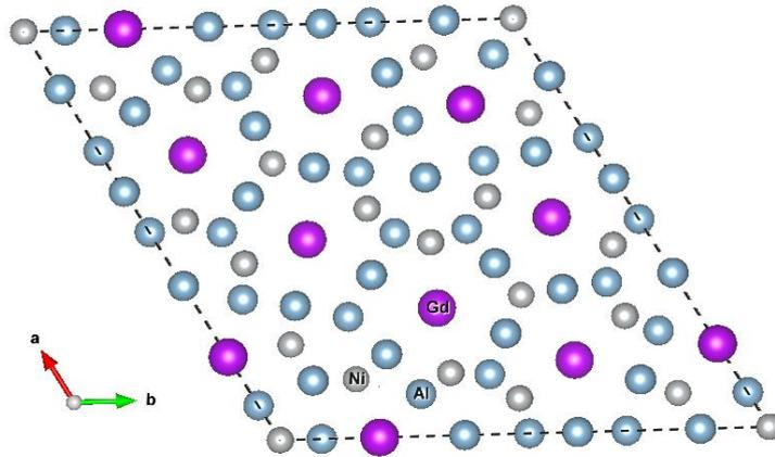
**Figure 1.** The crystal view of hexagonal  $Gd_3Ni_7Al_{14}$  compound.
