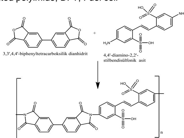
**Figure 1.** Synthesis of sulfonated polyimides (BPDA - DASDA)
