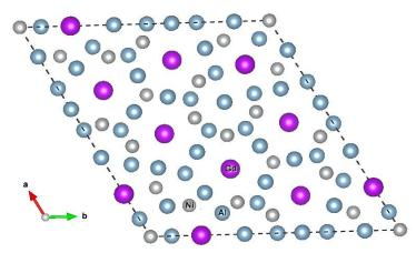
Figure 1. The crystal view of hexagonal Gd<sub>3</sub>Ni<sub>7</sub>Al<sub>14</sub> compound.
