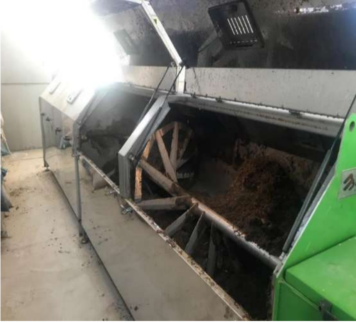
Figure 50. The Conversion Process of Organic Waste to Compost in the Waste Collection Center-2
